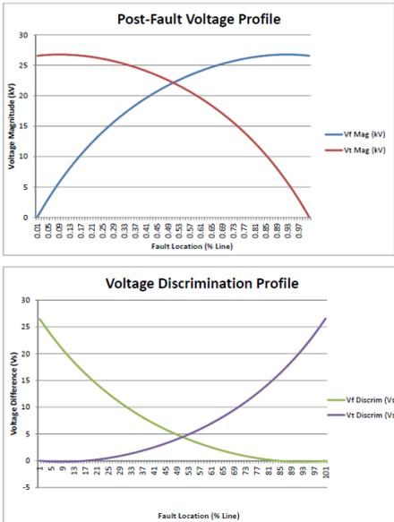
Figure 4: Voltage at relay location for sliding fault And voltage difference discrimination plot.
