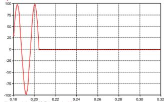
Figure 9: CVT with passive filter  $-V_{SEC}$
