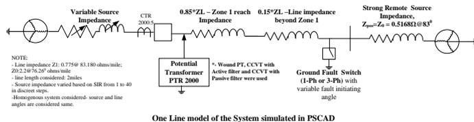
One Line model of the System simulated in PSCAD
