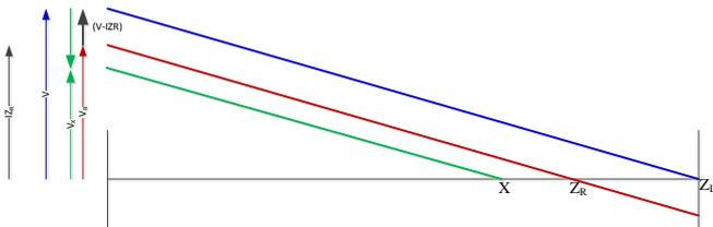
Figure 5: Phase relationship between V and (V-IZ<sub>R</sub>)
