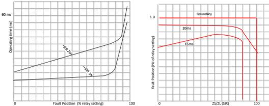
Figure 2: Typical Relay operating time-Constant Time Contour
