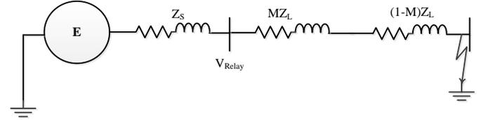
Figure 3: Single Line diagram showing Zone 1 Reach, M\*Z<sub>L</sub>
