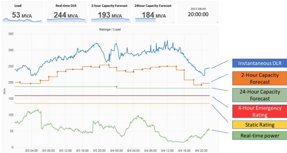
Figure 2: Transmission Capacity Forecast System Output showing 2- and 24-hour ahead forecasts
